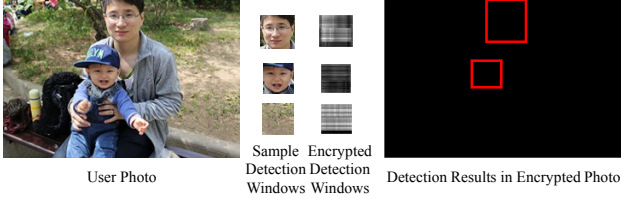
Figure 3: The secure face detection. The user photo are divided into detection windows, which are sent to the cloud one by one. The detection results are shown in rectangle.
